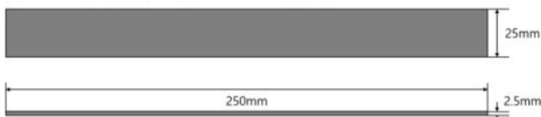
Fig. 3. Schematic diagram of tensile test according to ASTM D3039
