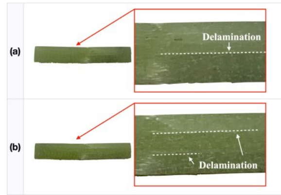
Fig. 8. Interlaminar shear strength of sensor embedded GFRP; (a) Neat GFRP, (b) Sensor fiber embedded GFRP, (c) FBG sensor embedded GFRP
