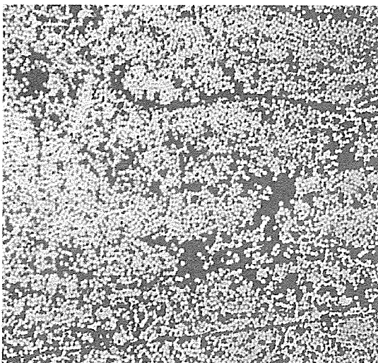
Fig.5. Micrograph of the composite made from commingled towpreg
