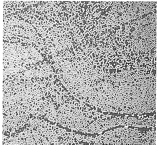
Fig.6. Micrograph of the composite made from powder coated towpreg
