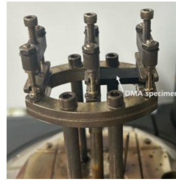
Fig. 4. Configuration of DMA test set-up
