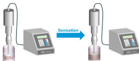
Fig. 1. Cleaning the spent coffee ground using an ultrasonic processor
