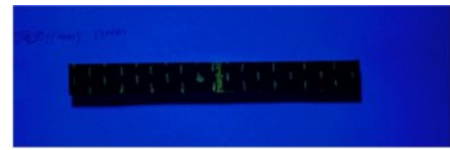
(a) Photograph of the specimen after spraying fluorescent liquid
