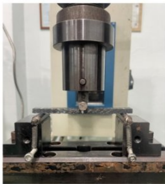
Fig. 3. 3-point bending test
