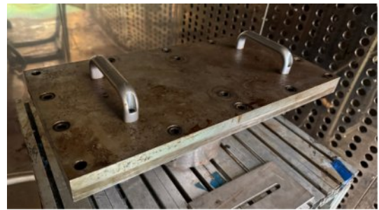
Fig. 2. Closed mold for RTM
