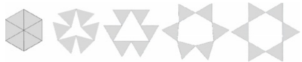
Fig. 2. Negative Poisson's ratio characteristic of TSP structures
