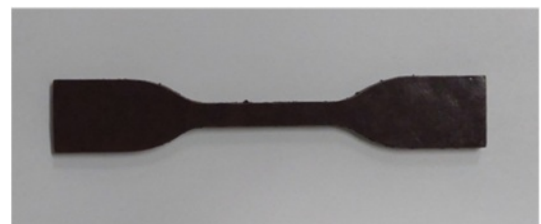
Fig. 2. ASTM D638 type IV specimen
