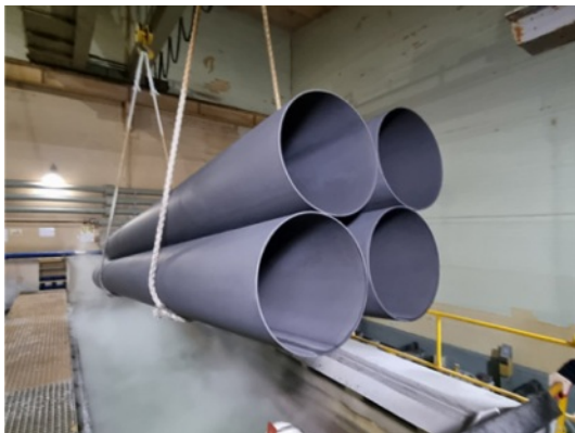
Fig. 5. Photo of steel pipe after chemical pretreatment
