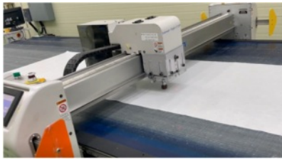
Fig. 9. Prepreg Cutting
