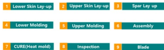
Fig. 2. Blade manufacturing sequence
