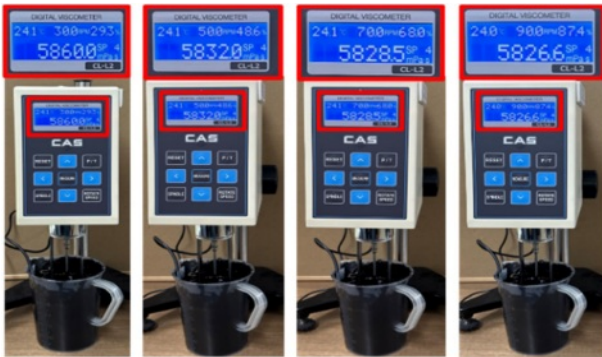
Fig. 5. Viscosity measurement of mixture for repair
