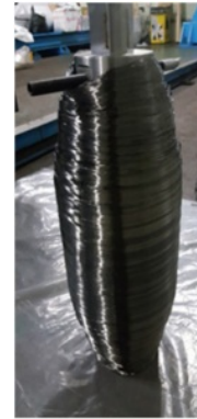
Fig. 2. Filament wound composite vessel
