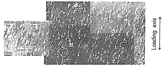
(a) N=5.70 \times 10^4 cycles, 2a=0.23\text{mm} , K_{\text{max}}=5.61\text{MPam}^{1/2}
