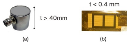
Fig. 1. Comparison of appearance between existing AE sensor (a) and MFC (b)
