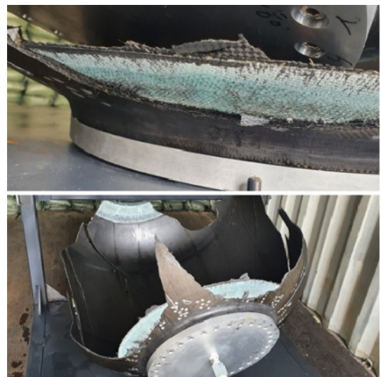
Fig. 16. Interface b/w the boss and the barrel after burst
