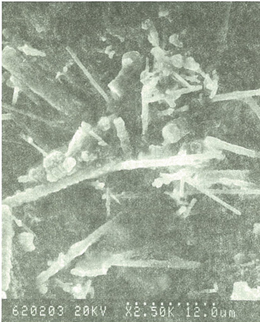
(a) Propagation along interfaces between interfacial compounds and matrix
