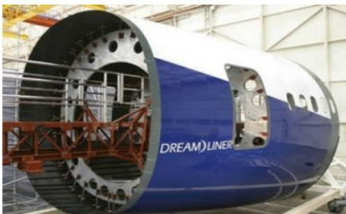
**Fig. 2.** Boeing 787 Dreamliner manufactured using CFRP. Reprinted with permission [8] Copyright 2022, ELSEVIER Ltd.
