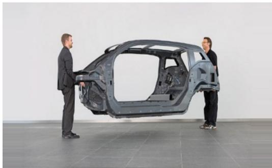
Fig. 4. Lightweight BMW i3 body. Reprinted with permission [18] Copyright, BMW
