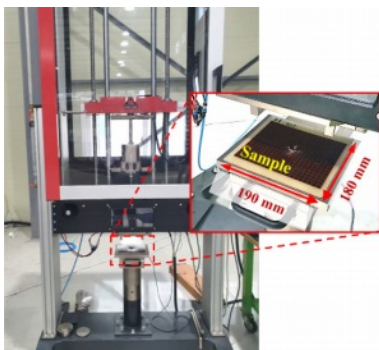
Fig. 6. Experimental setup of a low-velocity impact test for the fabricated RAS
