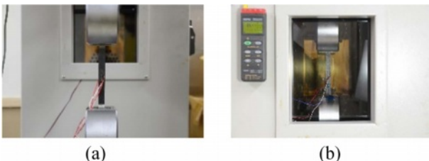
Fig. 4. Exposure environment for tensile test: (a) room temperature and (b) thermal environment in oven
