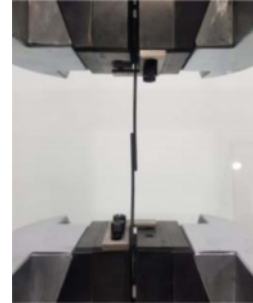
Fig. 7. Tensile test of joint specimen
