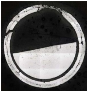
Fig. 7. Cross section of triplex SiC composite cladding (CVD SiC-SiC f /SiC-CVD SiC) after neutron irradiation [51]
