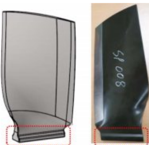
Fig. 1. Configuration of composite fan blade having dovetail joint element
