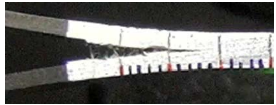
Fig. 9. Crack growth of DCB specimen
