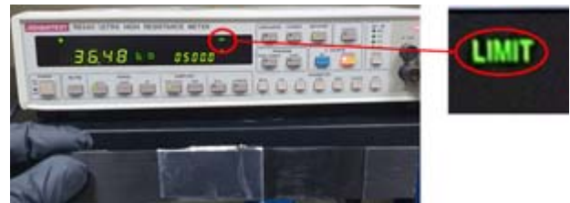
Fig. 6. Electric resistance of un-stitched single-lap joint measured by ultra high resistance meter
