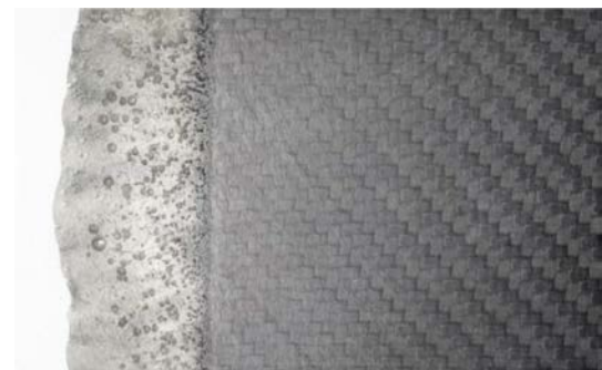
Fig. 13. Resin squeeze out effect
