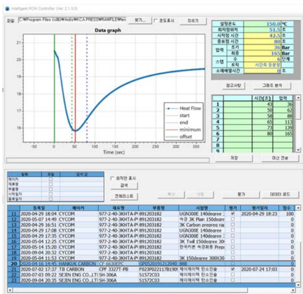
Fig. 4. PCM process control software
