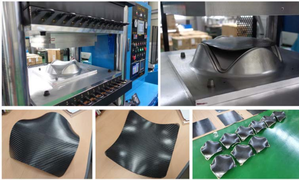
Fig. 14. 3D shape part molding results by K-3 process condition
