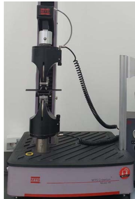
Fig. 10. 4-Point bending tester
