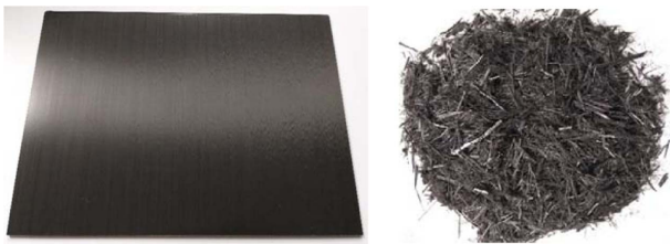
Fig. 5. Recycling test results of carbon fiber epoxy composites (left: CFRP plate, right: after shredding)
