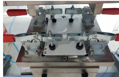
Fig. 2. Fixed specimen in drop weight test machine
