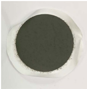
Fig. 2. Photograph of a rGO paper fabricated by vacuum filtration of rGO flakes dispersed in DMF
