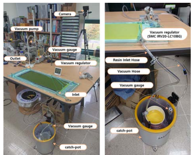
Fig. 4. Photograph of the VARTM process set-up
