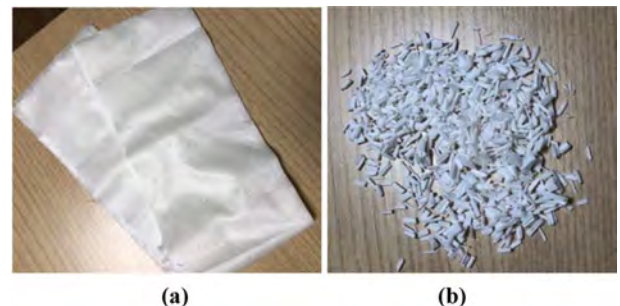
Fig. 2. Reinforcement for composites: (a) Nonwoven bamboo fabric and, (b) chopped bamboo fabric
