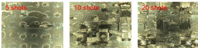
Fig. 6. Bonded surface of fractured specimen in shear test according to the number of laser shots
