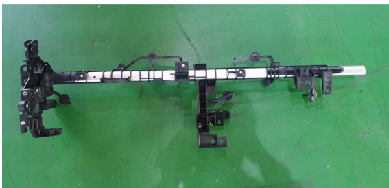
Fig. 4. A Cowl Cross Member with multi-material type (polymer+ aluminum bar)
