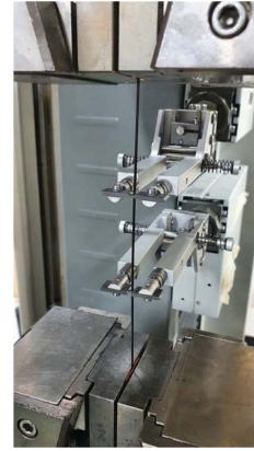
Fig. 4. Tensile test apparatus and specimen
