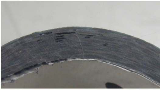
Fig. 1. Voids in the laminate
