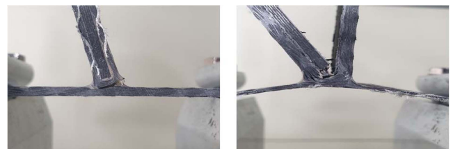
Fig. 15. Break behavior of 3D preform Beam Bending Test
