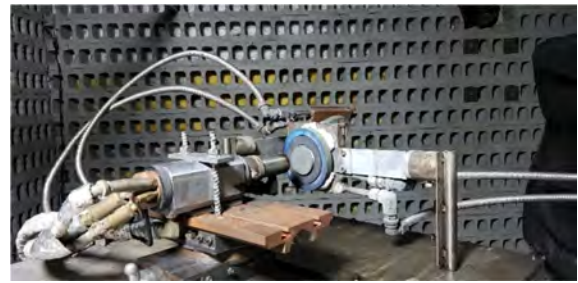
Fig. 3. The photograph showing burner test on SiC-coated C/C composite
