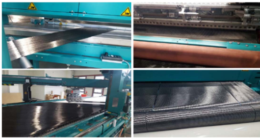
Fig. 6. Carbon NCF Fabric manufacturing process
