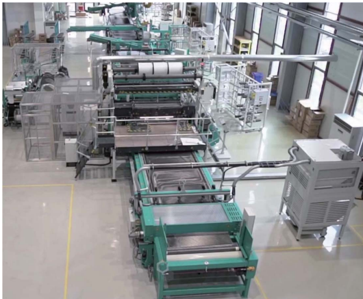
Fig. 3. Multi axial carbon fabric weaving machine(NCF)
