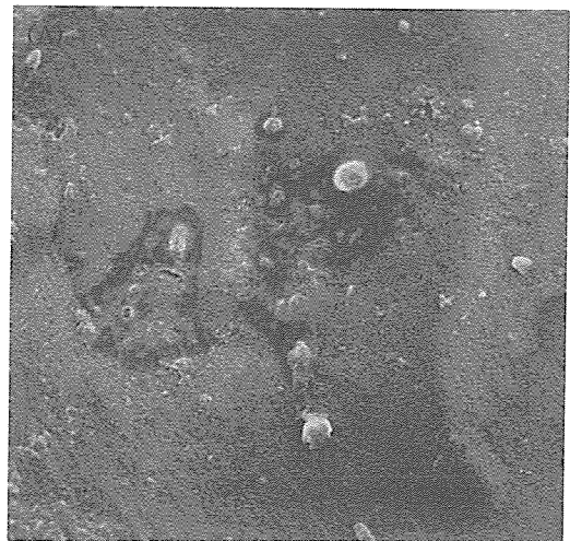
Fig. 8. SEM micrographs of BIS-GMA/silica with the variation of silica content ; (A) 10 wt% uncoated (B) 20 wt% uncoated (C) 15 wt% coated (D) 20 wt% coated. (X3000)
