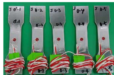
Fig. 3. Manufactured specimens of damped aluminum panel
