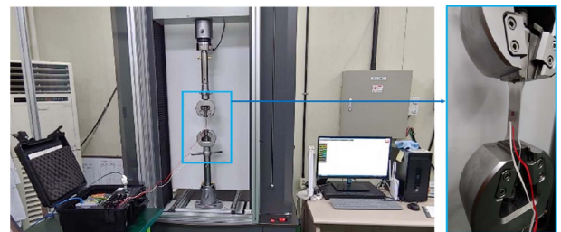
Fig. 2. Test set-up for tensile tests of damped aluminum panel
