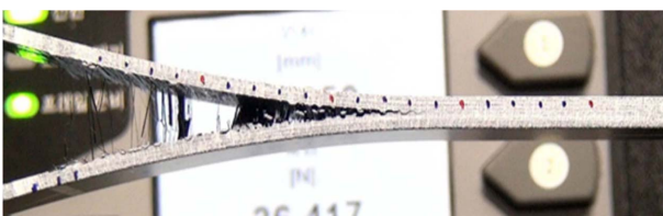
Fig. 4. Crack Propagation Shape during the Cross-ply DCB Test
