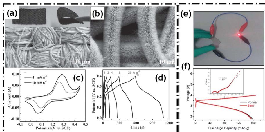
**Fig. 7.** (a,b) SEM image of NiCo NW on the CC (NCNW/CC), (c) cyclic voltammetry of the NCNW/CC (d) charge-discharge of the NCNW/CC from ref [54], (e) LED-on by LiCoO<sub>2</sub>//TiN, (f) charge-discharge of LiCoO<sub>2</sub>//TiN from ref [58]
