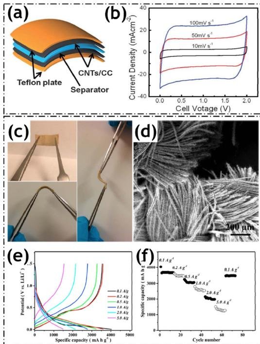
**Fig. 5.** (a) Schematic of CNT SC, (b) cyclic voltammetry of CNT SC from ref [46], (c) carbon-coated silicon NWs on the CF (c-Si NWs/CF), (d) SEM image of the c-Si NWs/CF, (e) charge-discharge of the c-Si NWs/CF, (f) rate capability with respect to cycle number from ref [47]
