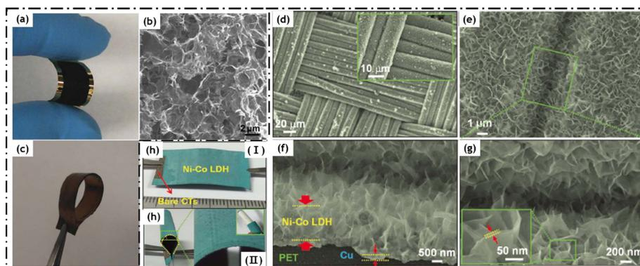
**Fig. 4.** (a) A functionalized graphene hydrogel (FGH) in the form of thin film, (b) SEM image of microstructures of the FGH, (c) a supercapacitor with the FGH from ref [41], (d-h) SEM images of the nickel-cobalt layered double hydroxide nanosheets on the textile substrate from ref [42]
