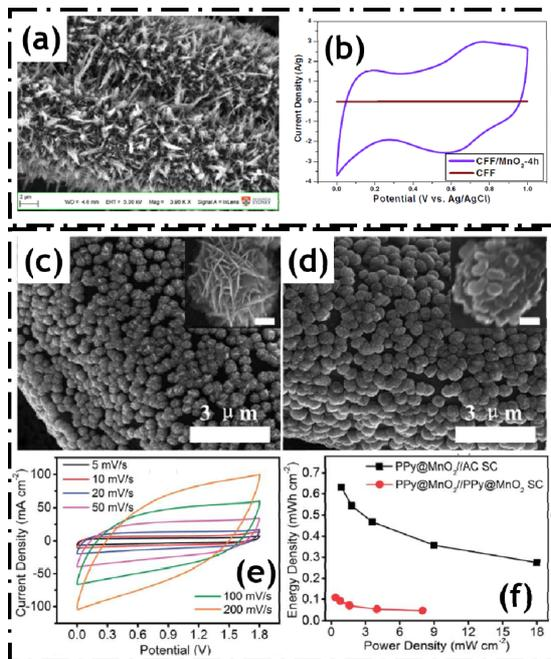
**Fig. 6.** (a) SEM image of Coral structure of  $\text{MnO}_2$  on the CF ( $\text{MnO}_2/\text{CF}$ ), (b) cyclic voltammetry of  $\text{MnO}_2/\text{CF}$  from ref [51], (c) SEM image of  $\text{MnO}_2$  nanoflower on the CC (MNF/CC), (d) PPY-wrapped MNF/CC, (e) cyclic voltammetry of the ASC, (f) ragon plot of the ASC from ref [52]
