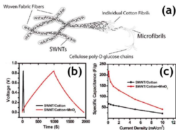
**Fig. 2.** (a) Schematic of cellulose fibers wrapped by SWNTs, (b) charge-discharge of the SWNT/cotton and the one with  $\text{MnO}_2$ , (c) Specific capacitance with respect to different current density from ref [38]
