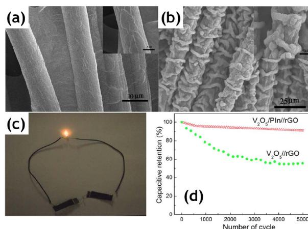
**Fig. 8.** (a) SEM image of reduced graphene oxide on the activated CC, (b) vanadium oxide on the activated CC, (c) LED-on by V<sub>2</sub>O<sub>5</sub>//Pin//rGO, (d) cyclic performance from ref [60]
