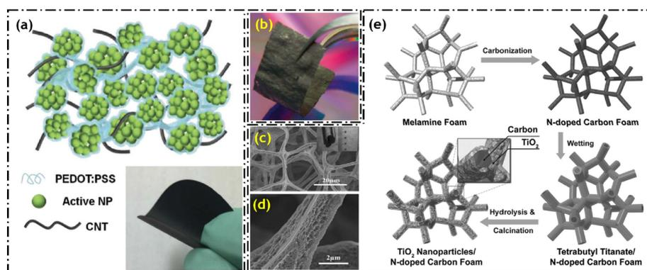
**Fig. 1.** (a) Schematic of active material, CNT and PEDOT:PSS composite from ref [25], (b) free-standing graphene paper from ref [31], (c) SEM image of N-doped carbon foam with  $TiO_2$ , (d) the magnified image, (e) Schematic of synthesis of the N-doped carbon foam with  $TiO_2$  from ref [32]
