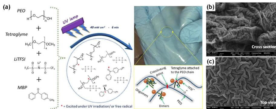
**Fig. 9.** (a) Schematics of preparation of interlinked solid polymer electrolyte (ISPE) and illustration (b, c) SEM images of ISPE from ref [64]
