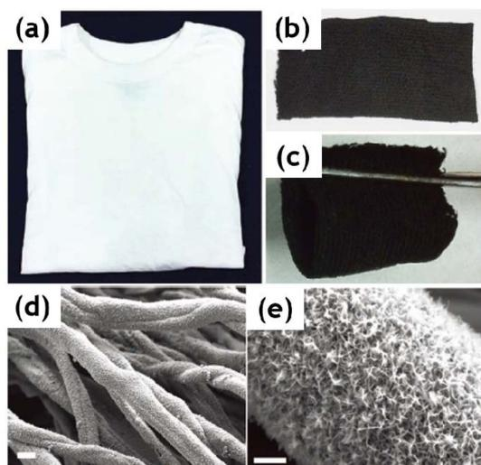
**Fig. 3.** (a) A commercial cotton T-shirt, (b, c) activated carbon textiles (ACT), (d, e) SEM images of the ACT coated with  $\text{MnO}_2$  from ref [40]
