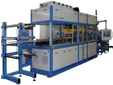
Fig. 2. Continuous compression molding (CCM) machine by Large
