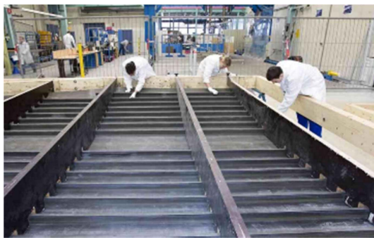
Fig. 1. A400M Cargo Door Fabrication using VAP Process [8]
