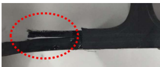
Fig. 11. Failure shape of composite T-Joint
