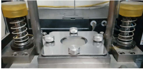
(b) Experimental setup for dropweight impact test
