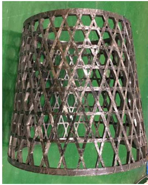
Fig. 4. Cone-type composite lattice structure
