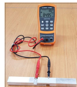
Fig. 6. Measurement of electric resistance by LCR meter
