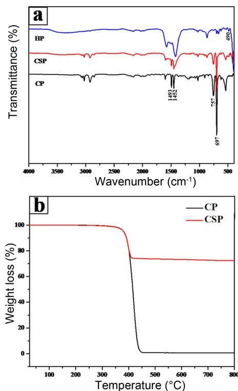
**Fig. 3.** (a) FT-IR spectra of PS core particles (CP), PS-ZnO core-shell particles (CSP) and ZnO hollow nanoparticles (HP). (b) Thermal degradation behavior of PS core particles (CP), PS-ZnO core-shell particles (CSP), and ZnO hollow nanoparticles (HP)
