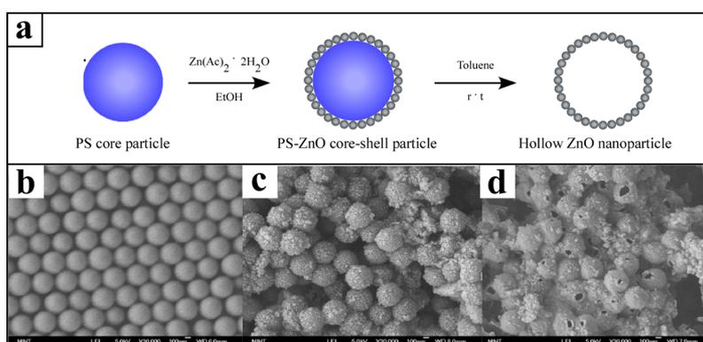
**Fig. 1.** (a) Schematic representation of the formation of ZnO hollow nanoparticles. SEM image of ZnO (b) PS core particles (CP) (c) PS-ZnO core-shell particles (CSP) (d) ZnO hollow nanoparticles (HP)
