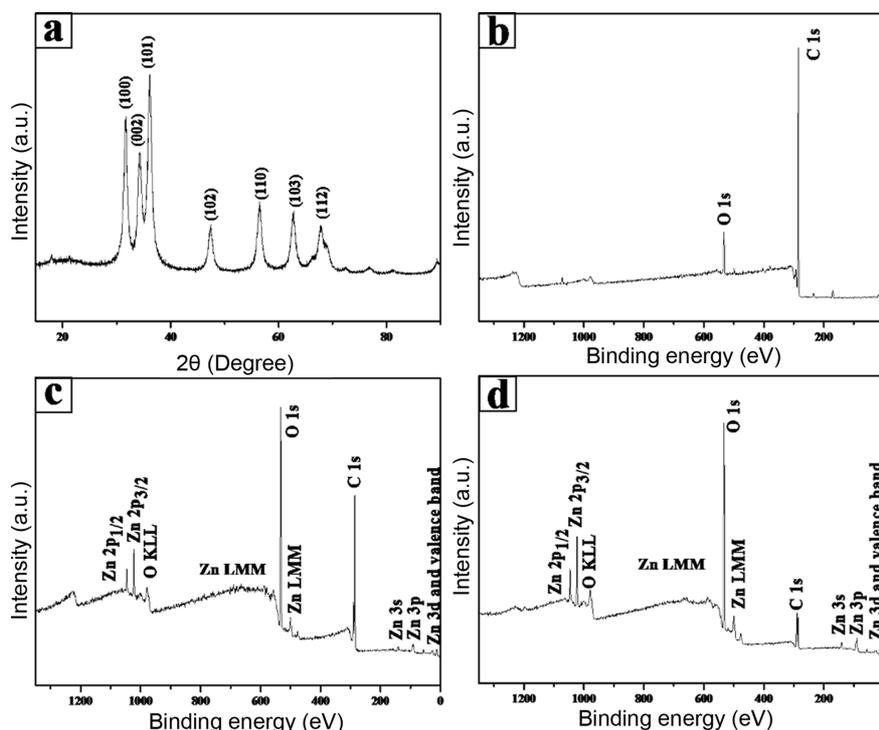
**Fig. 2.** (a) XRD pattern of the as-obtained ZnO hollow nanoparticles. XPS spectra of ZnO (b) PS core particles (CP) (c) PS-ZnO core-shell particles (CSP) (d) ZnO hollow nanoparticles (HP)
